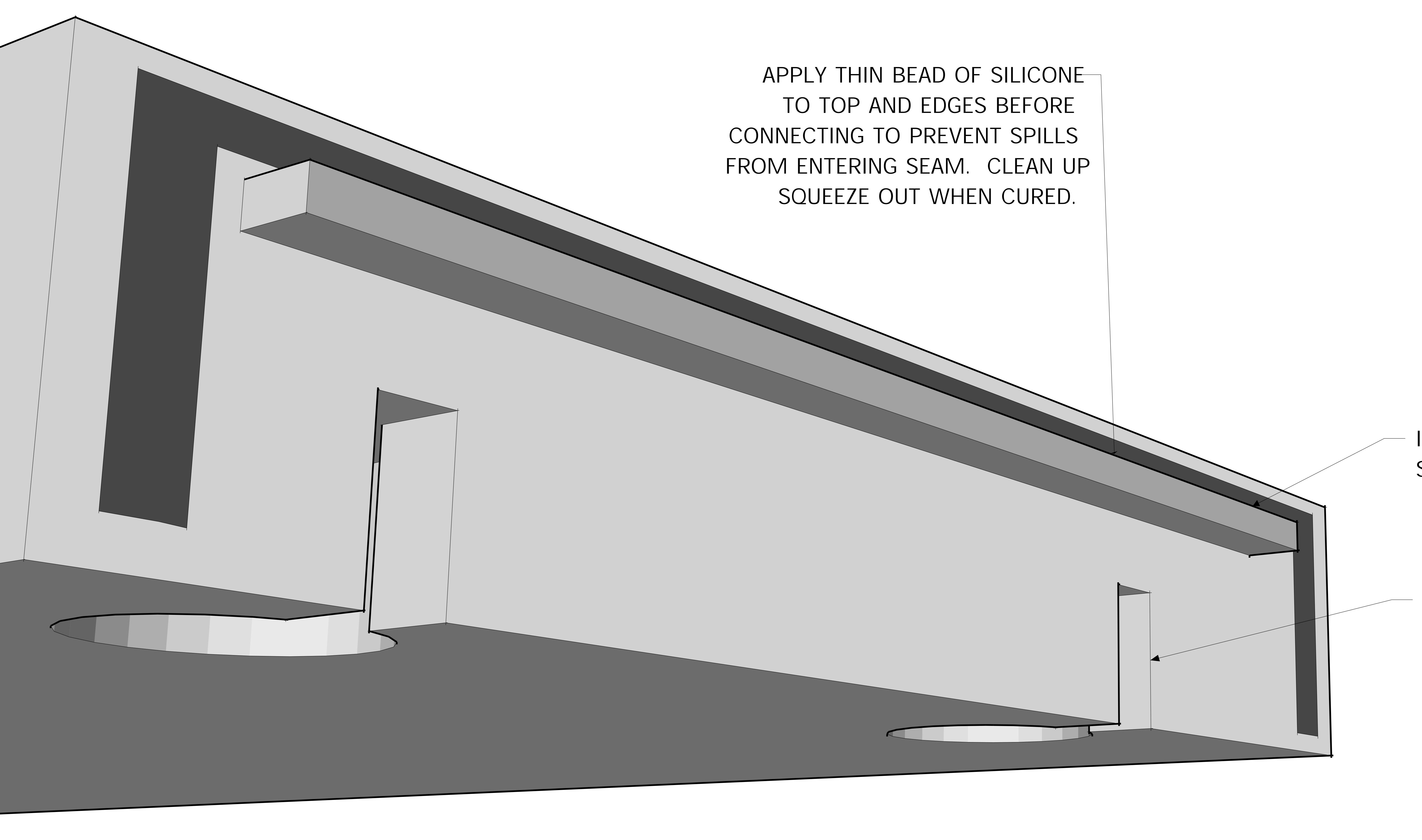
INSERT LOOSE SPLINE FOR GENERAL SLAB-TO-SLAB ALLIGNMENT
